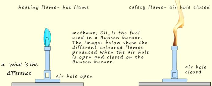
between complete and incomplete combustion? Incomplete combustion is combustion where there is a reduced amount of oxygen present. The products are flammable (soot and carbon monoxide) indicating that there is not enough oxygen present.
